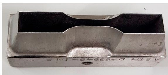
Figure 3. Dog-bone mold used to cut membrane samples used for dynamic mechanical analysis test.
