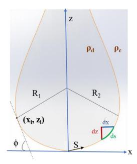
Figure 19. Schematic diagram of the characteristics of the pendant drop.
