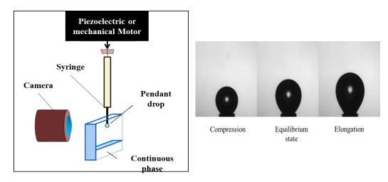
Figure 22. Close-up views of an oscillating drop.
