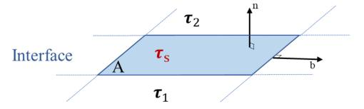
**Figure 4.** The surface element **A** separated two fluids denoted 1 and 2. The unit vectors normal and tangential to the surface are denoted by **n** and **b**, respectively.
