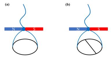
**Figure 1.** (a) Rayleigh's experiment involving a ring of thin brass wire placed on the surface of the water and dusted over with fine sulfur. The system was magnetically rotated using a magnetized sewing needle (NS). (b) A material diameter of the same brass wire was added to the ring. Reprinted with permission from Ref. [17]. Copyright 1890 Copyright Royal Society.
