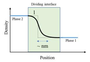
**Figure 3.** Schematic plot of the density  $\rho$  as a function of position x crossing the interface.
