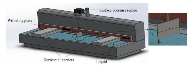
Figure 17. Schematic diagram of the Langmuir balance.
