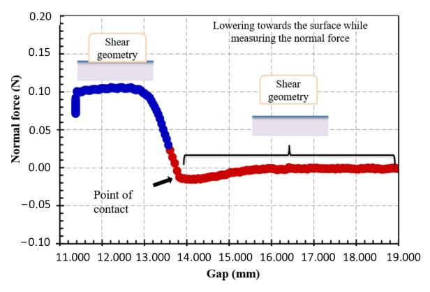
Figure 5. Positioning of the object at the interface with normal force assistance.
