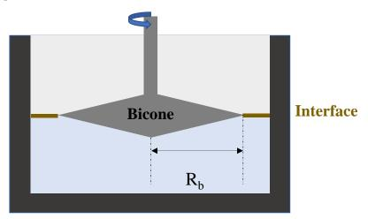
Figure 11. Profile section of the bicone device.
