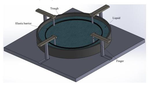
**Figure 18.** Schematic diagram of the radial trough setup composed of a circular Teflon trough with an elastic barrier and aluminum fingers, controlled by a stepper motor. Adapted from Ref. [27]. Copyright 1855 Copyright Taylor and Francis.
