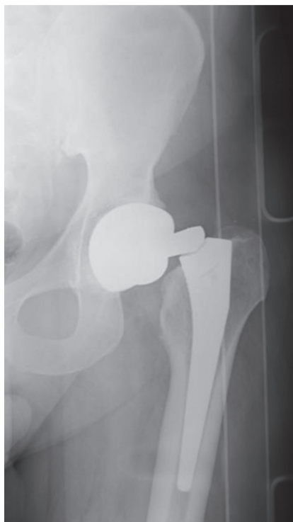
Figure 1a. Case 1. Left hip AP view radiographs showing a fracture of the modular neck at the stem-cone junction
