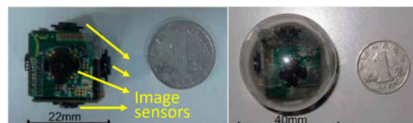
Figure 1. Prototype of the multiple cameras endoscopic capsule (MCEC), the print circuit board (PCB) cube with six image sensors, is sealed into a transparent biocompatible plastic shell for practical verification.
