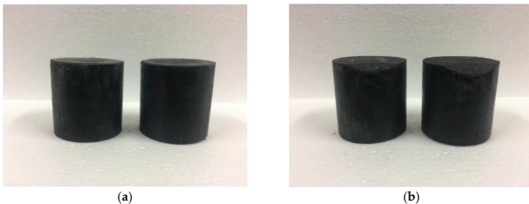
Figure 11. M–S–H cement-solidified body with 0.8 wt % \text{Cs}^+ before (a) and after (b) anti-shock testing.
