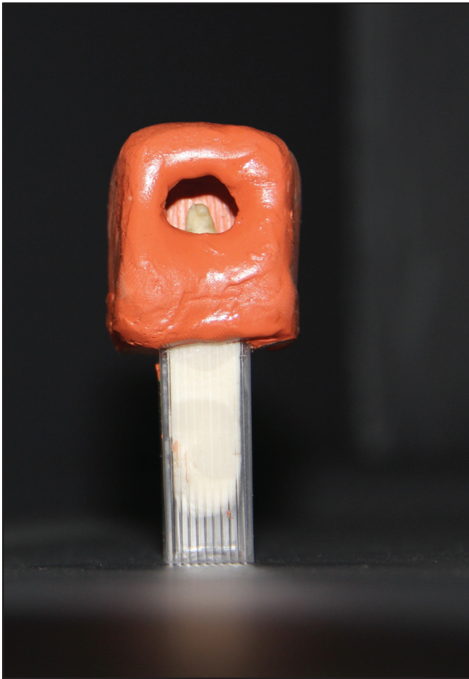
Figure 2. Simulated bony crypt used for resection and root-end preparation
