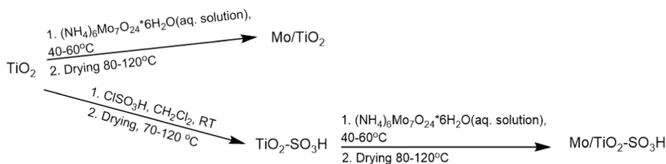
Figure 1. Scheme of the synthesis of catalysts based on titanium oxide.
