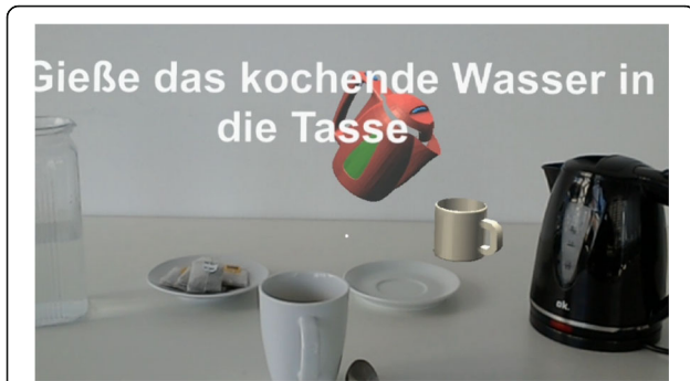
Fig. 1 Display of holographic cues presented by the Therapy Lens application on a Microsoft HoloLens. The subtitle and holograms indicate the first step in the tea making task of pouring the heated water into the mug (“Gieße das kochende Wasser in die Tasse”). The red kettle and the small white mug (on the right) are both holographic objects
