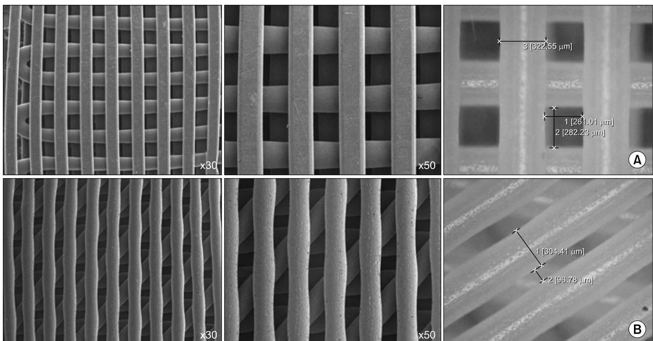
**Fig. 1.** Scanning electron micrograph images of  $90^\circ$  plotted polycaprolactone (PCL) 300/300 scaffold (A) and  $45^\circ$  plotted PCL 300/300 scaffold (B).
