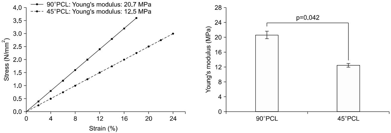
**Fig. 2.** Mechanical properties of three-dimensional printed polycaprolactone (PCL) scaffolds. Mean tensile stress, strain, and Young's modulus values of two different types of PCL scaffolds.
