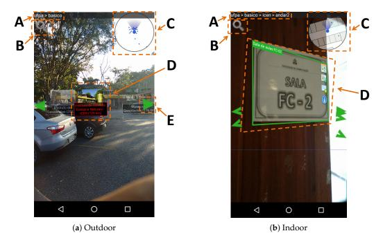
**Figure 5.** The graphical user interface of the prototype application:(**a**) the application running outdoors and following a route; and (**b**) the application running indoors and recognizing a room sign of a POI.
