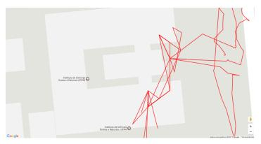
**Figure 14.** GPS based location when the participant is inside the ICEN. It is infeasible to use GPS in indoor environments with the tested GPS technology.
