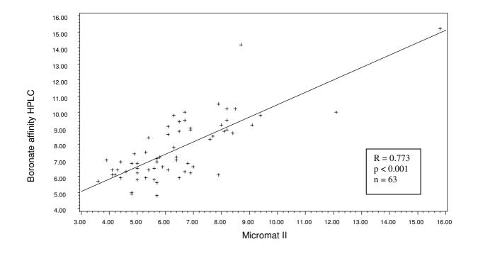
Figure I Scatterplot and regression line of HbA1c values produced from boronate affinity HPLC and Micromat II.
