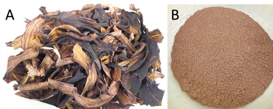
Figure 1. Waste banana peels and banana peel flour. A: Waste banana peels, B: Flour obtained from the waste banana peels.
