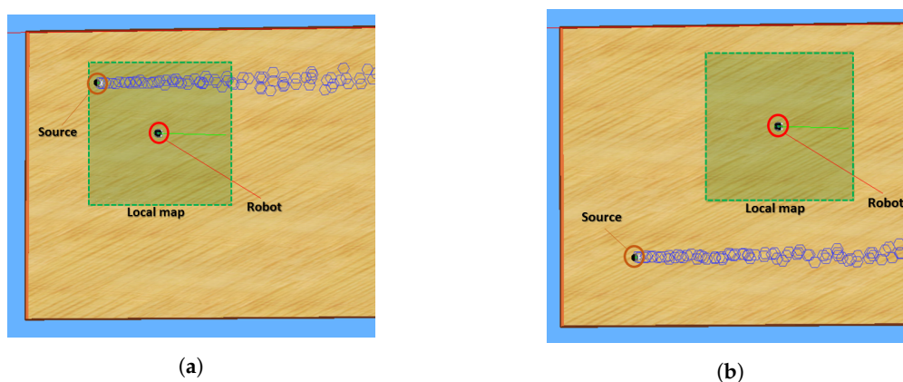
Figure 2. Position of the local map with respect to the source and the plume: (a) source inside the local map of the robot and (b) local map outside the plume.
