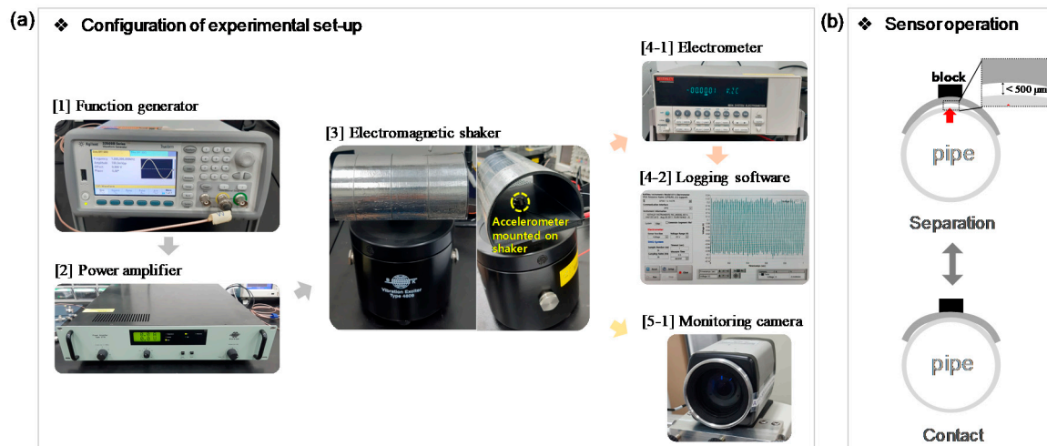
Figure 2. (a) Configuration of experimental setup. (b) Schematic illustration of the PVV sensor operation.
