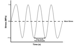
**Figure 3.** Sinusoidal pattern created by fully reversed loading. The sinusoidal pattern results from the alternation of tensile (reversal 1) and compressive (reversal 2) loading during cycling.
