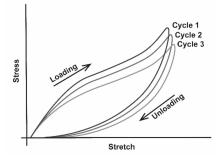
**Figure 5.** Theoretical example of hysteresis loops indicative of cyclic softening. Cyclic softening occurs when the peak stress of a material decreases with an increased number of cycles.
