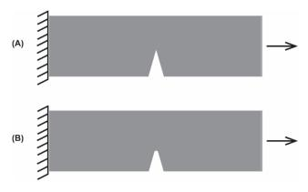
**Figure 6.** Theoretical examples of crack tips. (**A**) A sharp crack tip promotes rapid propagation of the crack. (**B**) A blunt crack tip slows the propagation of the crack.
