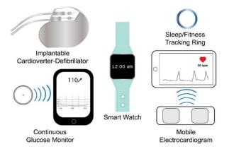
**Figure 1.** Examples of wearable sensing technologies. Wearable sensing technologies include internal (e.g., internal cardioverter-defibrillator and continuous glucose monitor) and external (e.g., smart watch, sleep/fitness tracking ring, and mobile electrocardiogram) wearable sensing technologies.
