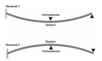
**Figure 4.** Example of a bending load. When a bending load is applied, the object experiences both tensile and compressive forces. During fully reversed cycling, the tensile and compressive forces alternate sides, resulting in the sinusoidal pattern observed in Figure 3.
