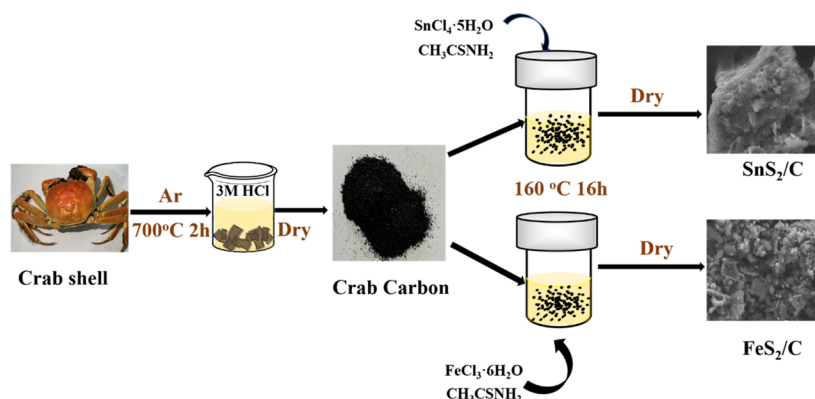
Figure 1. Schematic illustration of the fabrication process of the crab carbon and SnS 2 /C and FeS 2 /C composites.
