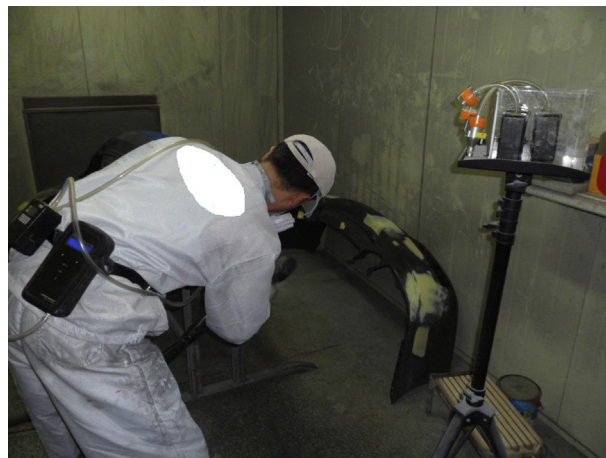
Fig. 2. The sanding process. For a single car bumper, 5 minutes of sanding and 15 minutes of painting is required.
