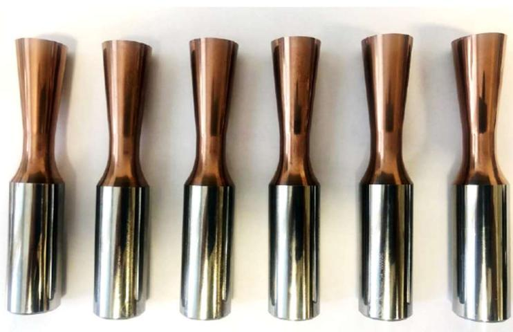
**Figure 6.** Monolithic rotary tools for forced rotation machining.
