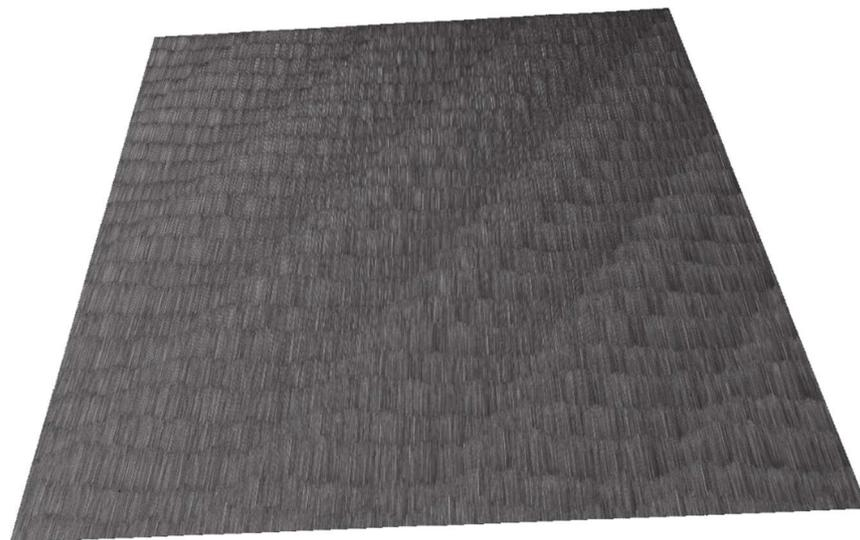
**Figure 12.** Optical surface texture measurement 42CrMo4 at cutting speed of  $300 \text{ m}\cdot\text{min}^{-1}$ .
