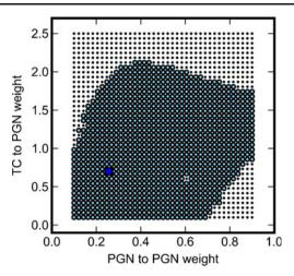
**Fig. 3** Stability of Model VI in two-dimensional space where the weights of connections from PGN to PGN and from TC to PGN are changed. *Small dots* denote negative samples, *larger circles* – positive samples (consistent with experiment). The *square* marks the parameters values shown in Table 5
