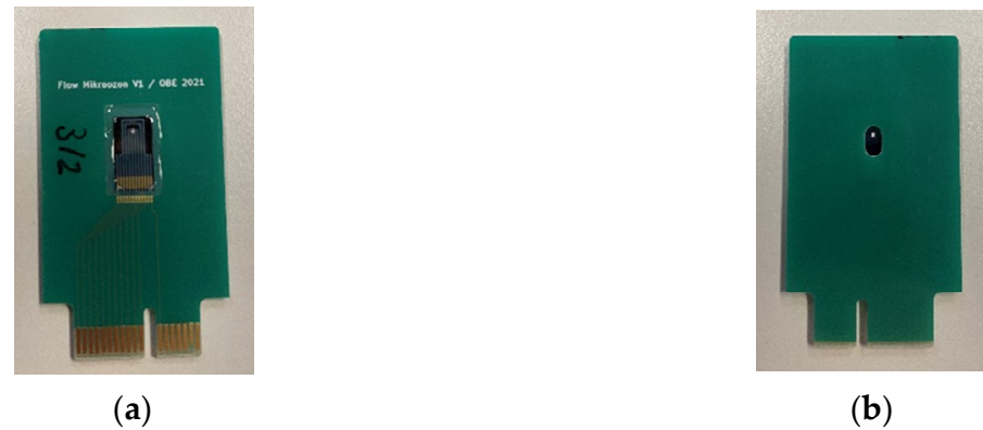
Figure 6. Sensor mounted on custom PCB: (a) top-view showing the sensor and card-edge connector and (b) bottom-view showing the hole below the PowderMEMS-modified backside cavity.
