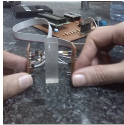
Figure 9: Test on glucose solution in transmittance mode
