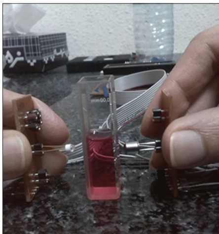
Figure 10: Test on artificial bilirubin solutions in transmittance mode
