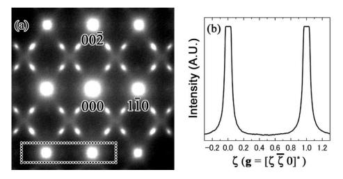
**Figure 7.** (a) SADP of the Zr-14 at.% Nb alloy (zone axis of [110]); (b) intensity profile along [110].
