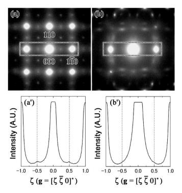
**Figure 6.** SADPs of the Zr-14 at.% Nb alloy: (a) SADP showing the zone axis of [001]; (b) SADP showing the systematic condition; (a',b') corresponding intensity profiles for the respective areas enclosed in the dotted boxes.
