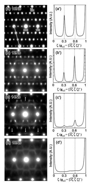
**Figure 3.** Results for Zr-x at.% Nb alloys ( $10 \le x \le 18$ ), as obtained by applying the incident beam in the [113] direction at room temperature: (**a**–**d**) diffraction patterns for x = 10, 12, 14, and 18, respectively; (**a**′-**d**′) corresponding intensity profiles.
