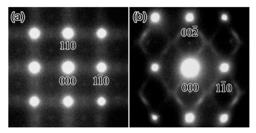
Figure 8. Diffraction patterns of Zr-18 at. %Nb alloy. The zone axis is [001] in (a) and [110] in (b).
