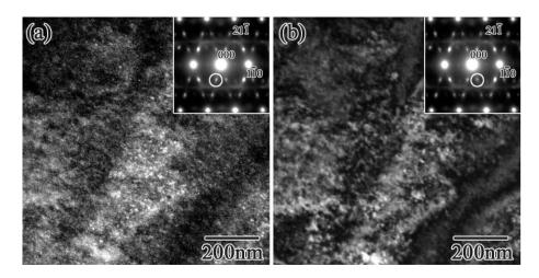
**Figure 5.** Dark-field images of Zr-14 at.% Nb alloy were observed by a circle in diffraction patterns in (**a**,**b**), respectively.
