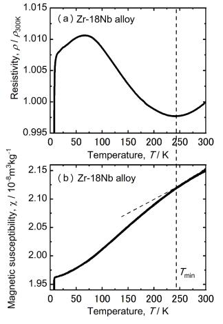
Figure 11. Electrical resistivity (a) and magnetic susceptibility (b) of the Zr-18 at.% Nb alloy.
