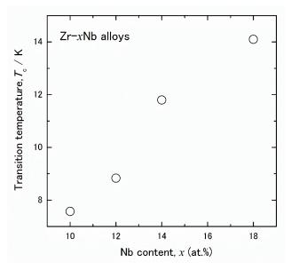
**Figure 2.** Nb content dependence of the superconductive transition temperature ( $T_c$ ) of Zr-x at.% Nb ( $10 \le x \le 18$ ) alloys.
