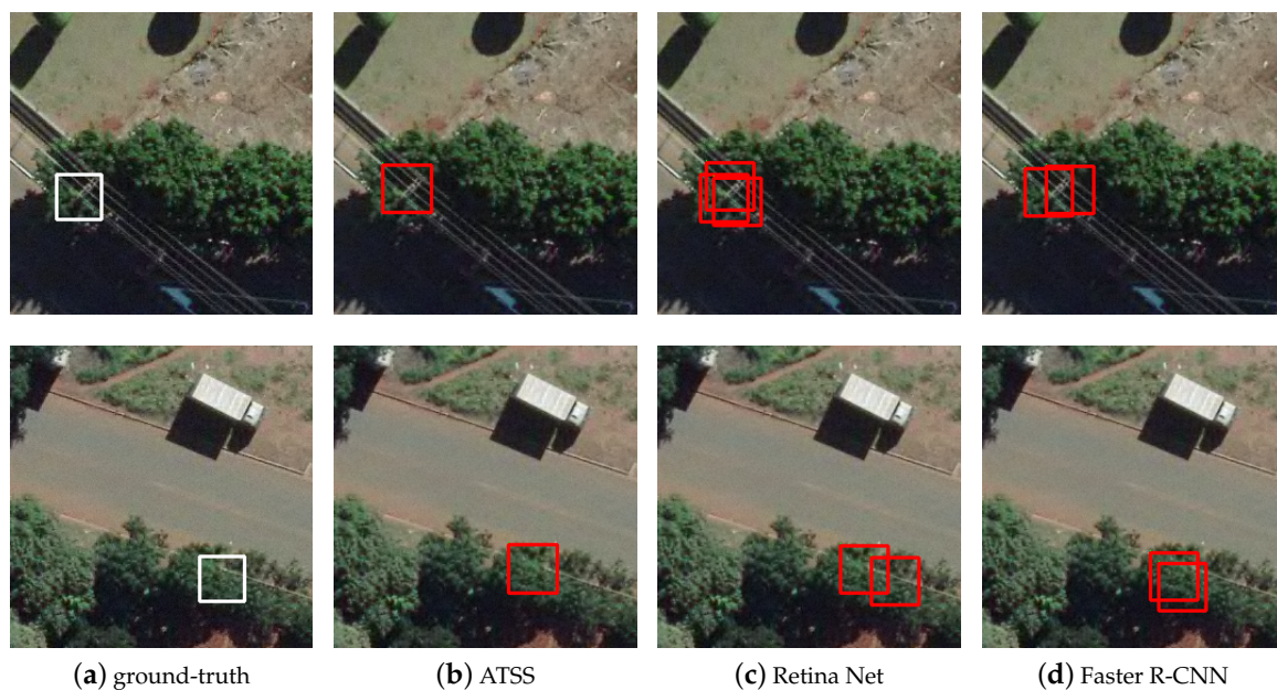
Figure 5. Results obtained by the methods when locating utility poles occluded by trees tops: (a) the ground-truth; (b) ATSS; (c) RetinaNet; and (d) Faster R-CNN.
