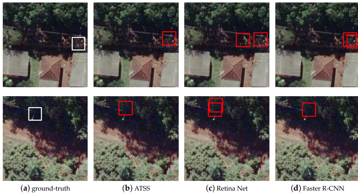
Figure 6. Examples of images with shaded poles: (a) ground-truth; (b) ATSS; (c) RetinaNet; and (d) Faster R-CNN.
