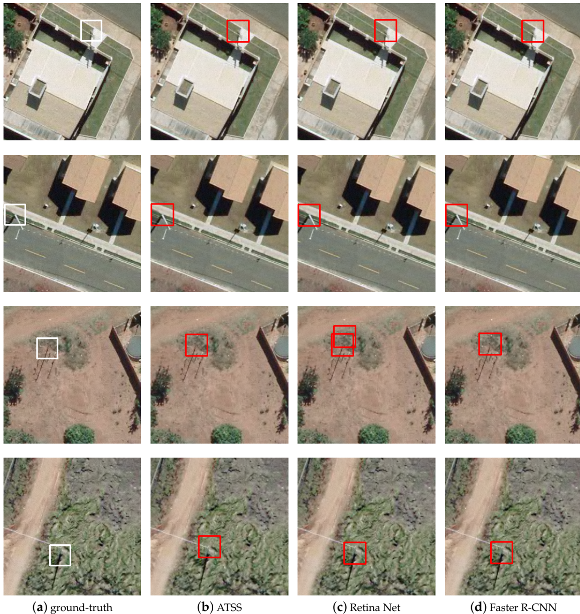
Figure 8. Examples of images with utility poles in different types of terrain: (a) ground-truth; (b) ATSS; (c) RetinaNet; and (d) Faster R-CNN.
