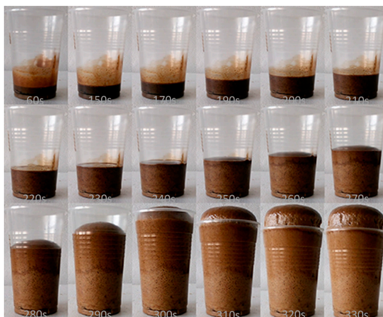
Figure 3. Foaming process of RPUF-D prepared from unfiltered BBPs without neutralization by sodium hydroxide.
