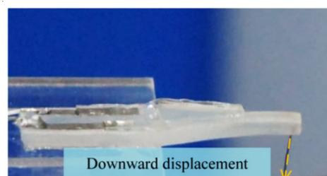
**Figure 10.** Photo of displacement applied to the tactile sensor.
