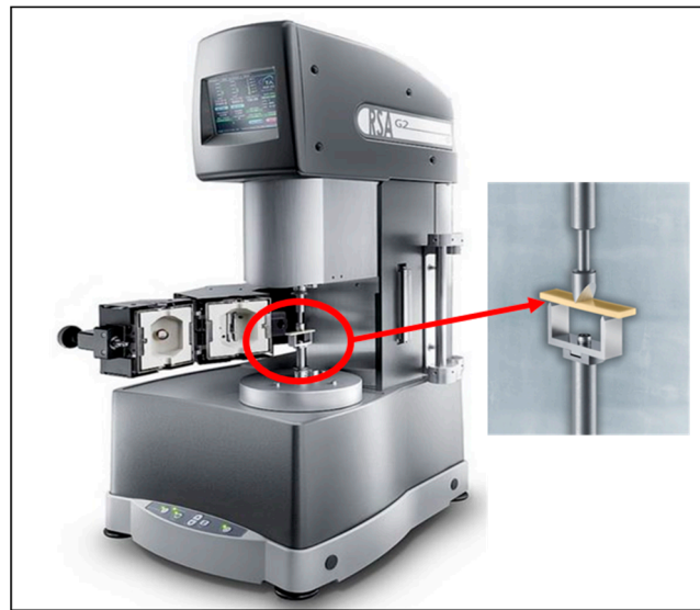
Figure 1. Dynamic mechanical Analyzer for three-point bending creep Analysis.
