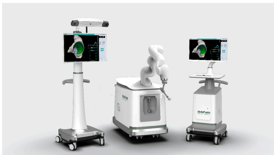
Figure 1. The robot console and the surgical platform of the LANCET robotic system.
