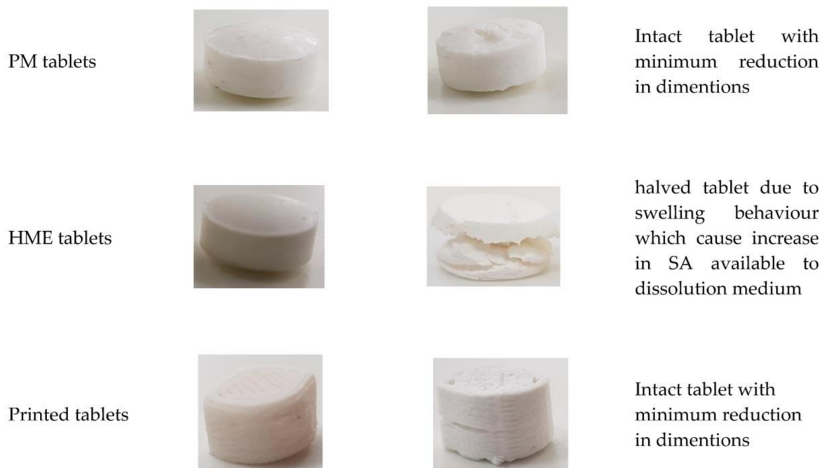
Figure 6. Visual changes to the shape of tablets (F2) after and before dissolution test.
