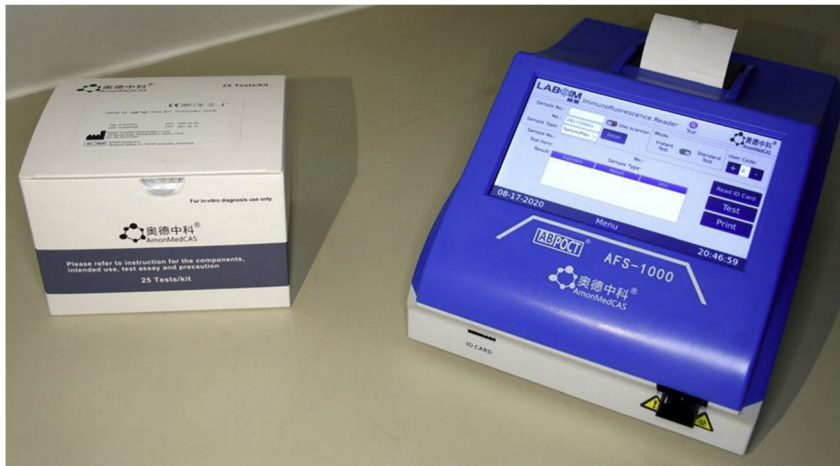
Fig. 1. The AmonMed assay test kit and the associated reader. It should be noted that the test cartridges of some batches did not fit into the reader, and therefore the evaluation had to be done with the naked eye.
