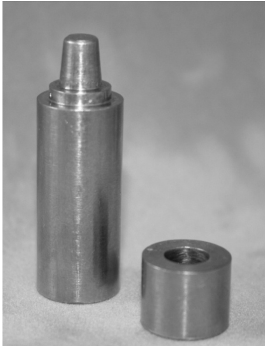
Fig1. Left, metal die used for veneering and right, template with certain inner diameter used for core wax-up
