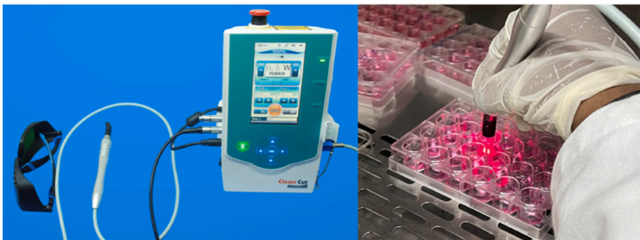
Fig. 3. Lllt device and irradiation on cultured titanium discs.
