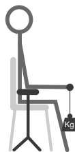
Figure 4. Position of the subject performing the load experiment. The elbow is placed on an armrest, and the load was increased from 0 kg to 5 kg every 10 s.
