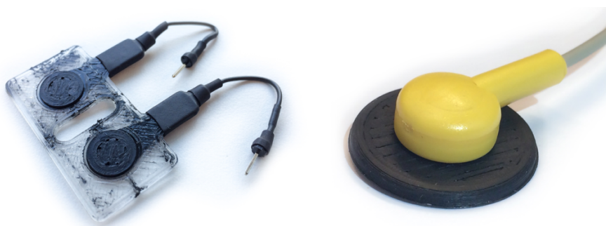
Figure 2. (Left): 3D-printed and assembled sensing structure (D10_IED20). (Right): Connected 3D-printed snap electrode.
