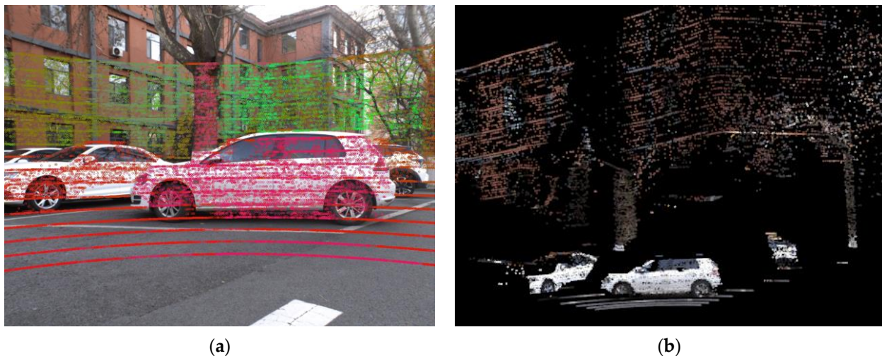
Figure 14. Fusion of image and upsampled point cloud using calibration results. (a) Projection from point cloud to image; (b) Image color rendering of the point cloud.
