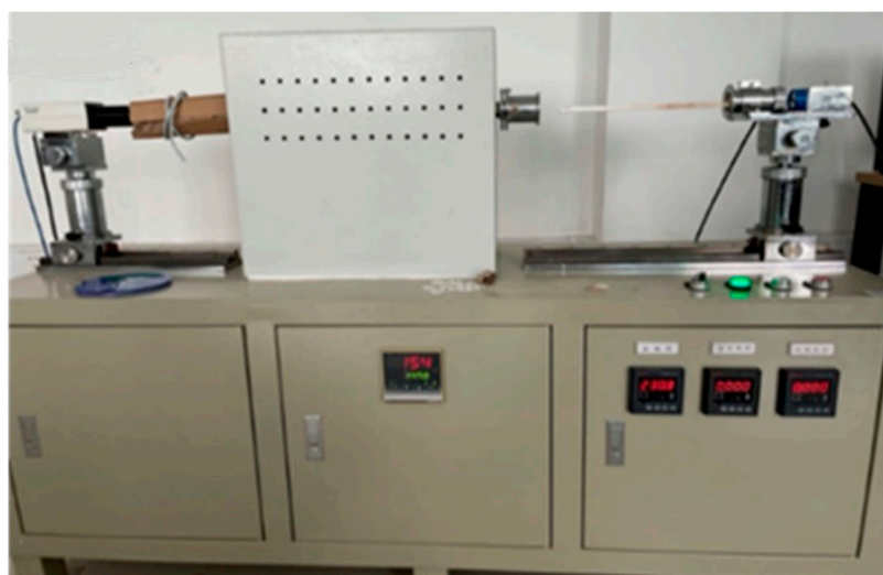
Figure 2. Test facility for determination of slag melting behavior.
