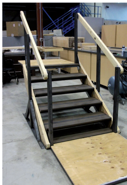
Figure 2. First full-scale prototype of the ARISE. It is inherently a conventional staircase but each end of the staircase also can operate as a platform lift.
