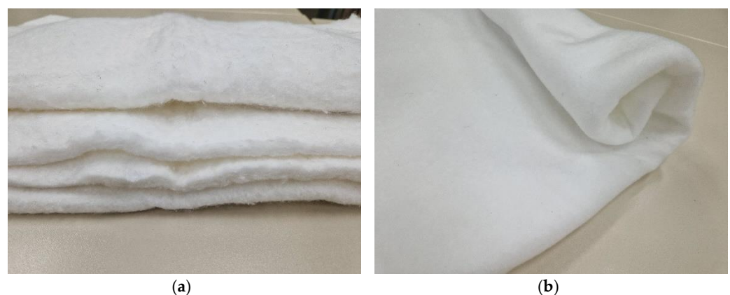
Figure 4. The nonwoven mulches produced by (a) viscose and (b) PLA nonwoven mulches.
