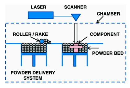
**Figure 1.** Illustration of the SLM process [5].
