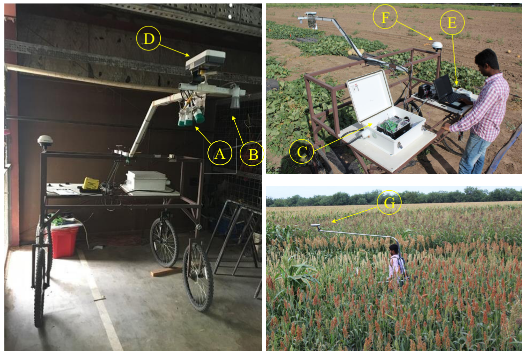
Figure 2 Configuration of sensors on the push-wheel sensing cart. (A) Three Apogee radiometers to pointing at different angles to measure canopy temperature. (B) An ultra-sonic sensor to measure canopy height. (C) CR3000 data logger housed in an enclosure to record data from radiometers and the ultra-sonic height sensor. (D) ACS-430 Crop Circle sensor to measure canopy vegetation indices. (E) GeoSCOUT Datalogger to record Crop Circle sensor data. (F) Hemisphere 101 GPS receiver with the signal-splitting cable connecting to the CR3000 and GeoSCOUT dataloggers. (G) A detached ACS-Crop Circle sensor mounted atop a backpack sensing frame (along with the GeoSCOUT Datalogger) for measuring tall vegetation. Photo credit: Xuejun Dong. Full-size DOI: 10.7717/peerj.12005/fig-2
