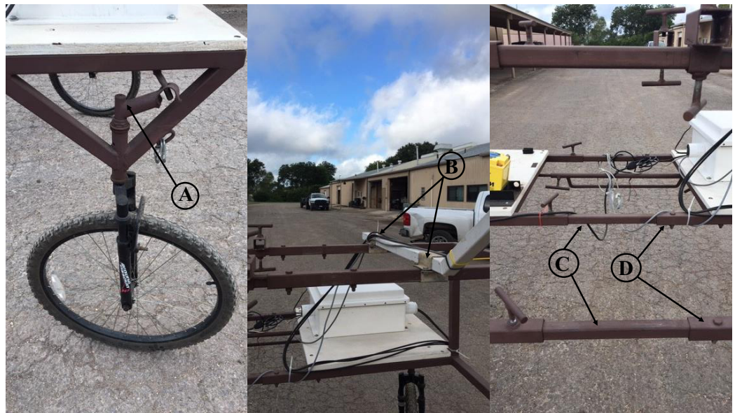
Figure 1 Highlights of the design features of the push-wheel sensing cart. (A) The rear wheels are installed with a steering mechanism to facilitate cart movement along a slightly curved row line as seen in a center-pivot field. (B) The sensor-mounting arm is fixed to the cart frame by two adjustable brackets, allowing flexible placement of the sensor-mounting arm along the width of the cart. (C) The smaller-sized tubings fitted into larger-size ones (D) to allow the width of the cart ( i.e. , the distance between the left and right side wheels) to be adjustable from 152 cm to 203 cm, a feature useful for measuring crops with different row spacings. Photo credit: Shane Sieckenius.
