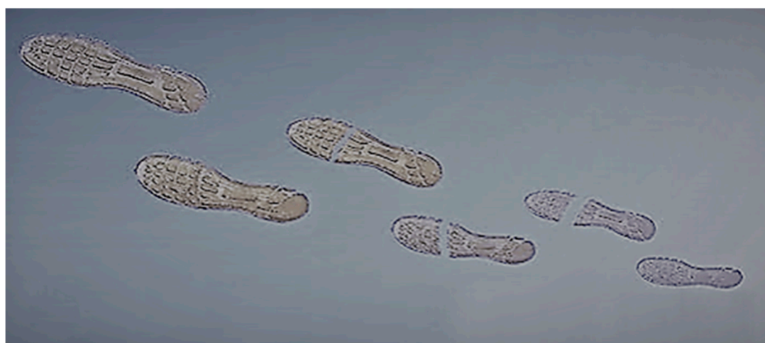
Figure 14. Severed 3D-printed shoe pad self-healing itself. (Adapted from [67]).
