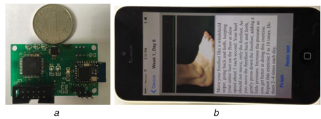
Fig. 2 Rehabilitation training system for foot exercises a Picture of the whole device b App and the GUI
