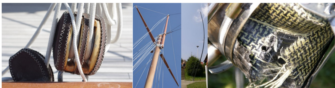
Figure 1. The classical wooden tackling versus the flexible composite mast is made from the polymer reinforced with aramid and carbon fibres.
