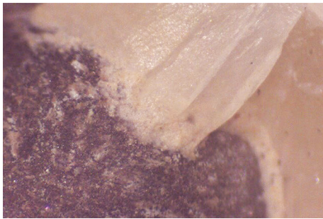
FIGURE 8: Stereomicroscopic images of the fractured crowns showing combined adhesive-cohesive mode of failure at 35x magnification.
