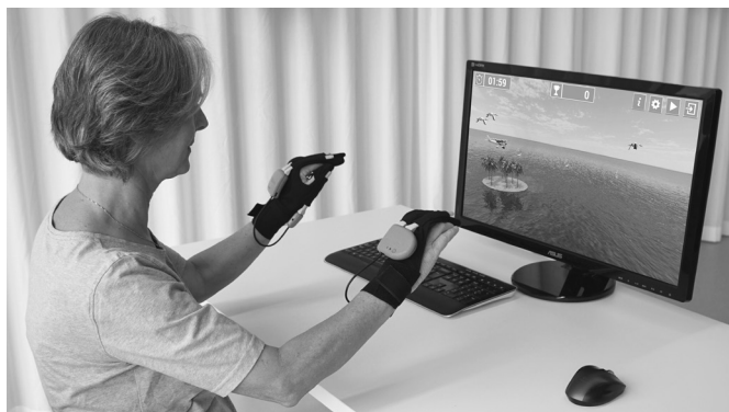
Figure 1 Virtual reality training system setup (Bi-Manu-Trainer, Reha Stim Medtec AG). The model wears wireless hand gloves with movement sensors attached. The screen displays real-time hand and finger positions.
