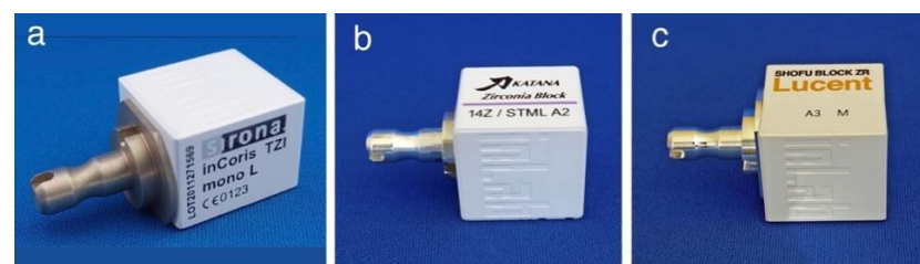
Figure 5. Zirconia CAD/CAM blocks for SpeedFire ® . (a) inCoris TZI ® (Dentsply Sirona, 3Y); (b) Katana ® Zirconia Block STML (Kuraray Noritake Dental Inc., M5Y); and (c) Shofu Block Zr Lucent ® CEREC (Shofu Inc., M4Y).
