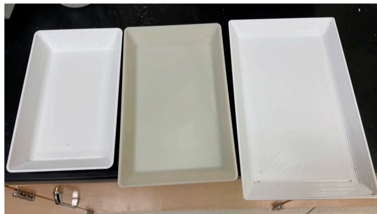
Figure 6. 3D-printed rectangular trays with one optimized thickness (middle, 1.56 cm) and two non-optimized thicknesses (left 2.00 cm and right 1.20 cm).
