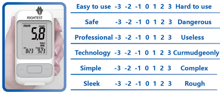
Fig. 5. Sample questionnaire design for a semantic differential method questionnaire on home glucose meters for the older adults.
