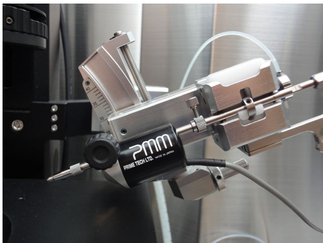
FIGURE 1 Drive unit of a Piezo-micromanipulator PMM4G (Prime Tech Ltd., Ibaraki, Japan) attached to TAKANOME® (MTK-1-03, NARISHIGE, Tokyo)
