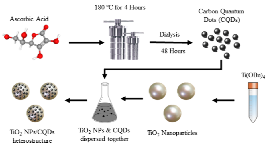
Figure 7. Synthesis of CQDs/TiO 2 Composite for MB degradation modified and reprinted from Ke et al. work. 56 Copyright 2017, Elsevier
