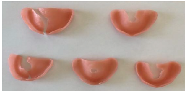
FIGURE 15: Triplex Hot® prosthesis bases subjected to pH 4 after fracture.
