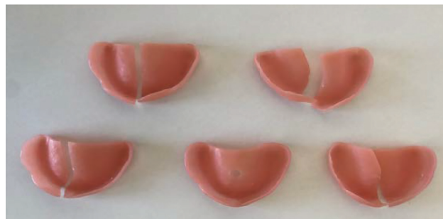
FIGURE 19: Megacryl® prosthesis bases subjected to pH 4 after fracture.
