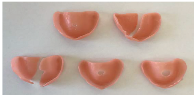
FIGURE 16: Triplex Hot® prosthesis bases subjected to pH 7 after fracture.
