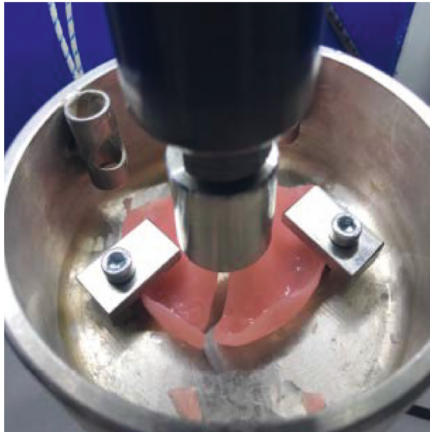
FIGURE 10: Prosthesis base fracture.
