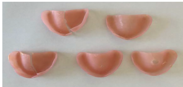
FIGURE 17: RS Vertex® prosthesis bases subjected to pH 7 after fracture.
