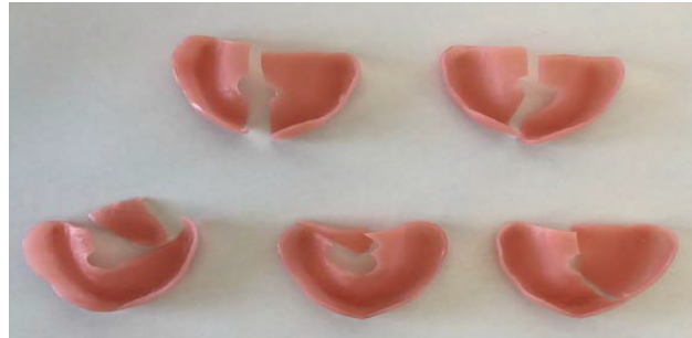
FIGURE 14: Megacryl® prosthesis bases subjected to pH 7 after fracture.
