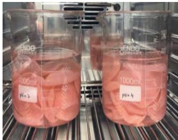
FIGURE 6: Prosthesis bases subjected to different pH values (pH 4 and pH 7).
