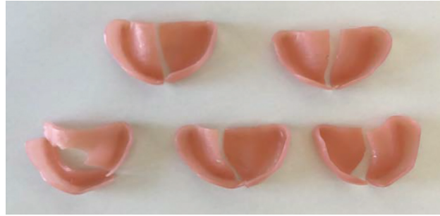
FIGURE 18: RS Vertex® prosthesis bases subjected to pH 4 after fracture.
