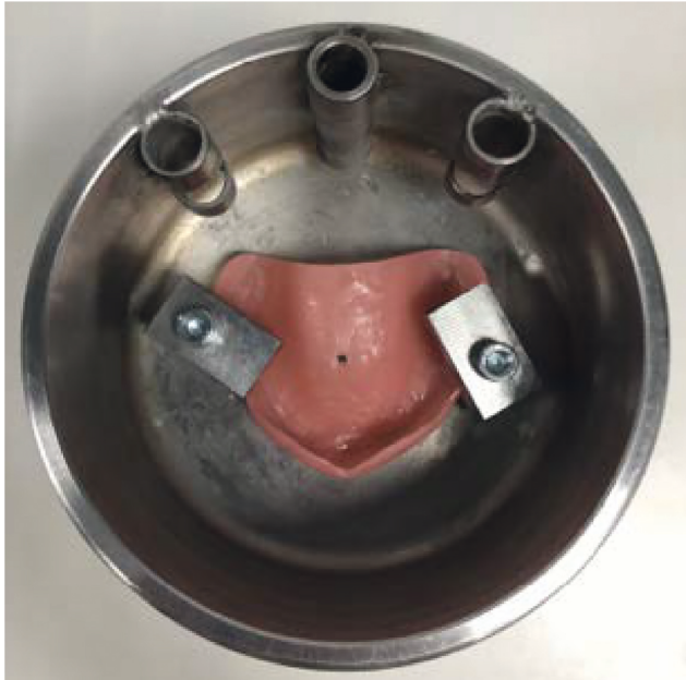
FIGURE 8: Prosthesis base placed to test the impact resistance. A point was marked at the center of the palate.
