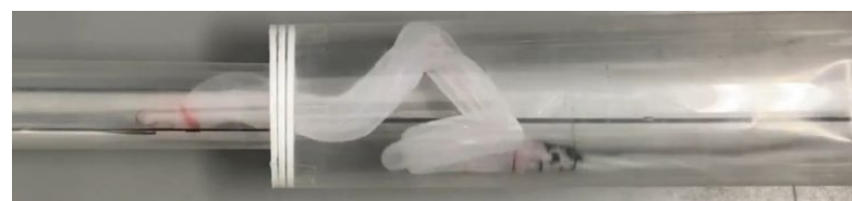
Figure 15. Experiment using a biased pitch device in a horizontally fixed pipe with the same diameter as that of the 50A and 20A pipes. (a,b) depict the device driven by an air pressure of 0.10 MPa and 0.15 MPa, respectively.
